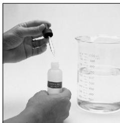
Step 3: Using caution not to touch the arrow end of the glass titrator tube (to avoid contamination), insert the tube all the way into the metal snapper and break off the end.
