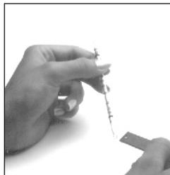
**Do not touch arrow end of titrator tube with fingers.**
