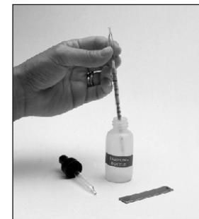
Step 5: Wait approximately one and one-half minutes or until the solution has wicked-up (capillary action) to the top of the titrator tube. The cotton at the top of the tube will change color to amber when fully saturated.
