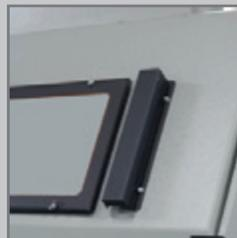
Each Marco Blast Cabinet includes a mylar window cover dispenser. Replaceable mylar window film protects the glass viewing window from abrasive rebound.
