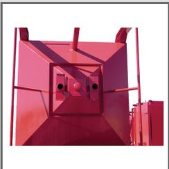
725 Cu. Ft. Abrasive Storage Hopper includes rain guards, shedding water and preventing rain from entering the abrasive blasting pot.
